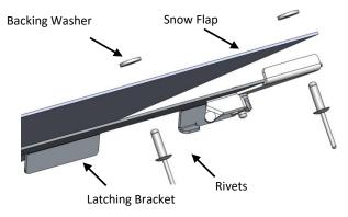
Rivet orientation is critical! Rivets MUST enter from bracket side and out snow flap side. Included rivet washers MUST be used. Install middle 2 rivets first, followed by the
